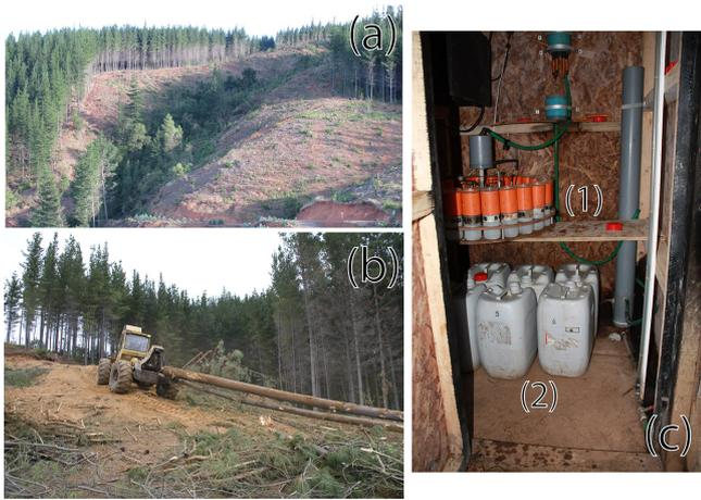
**Figure 2.** Pictures showing the experimental catchments, the logging procedure, and the suspended sediment monitoring devices. (a) Rainy season logged watershed (watershed 3) in the subsequent dry season (March 2010). (b) Skidder dragging logged stems uphill to the next landing in watershed 3. (c) Custom-built sediment sampling system: (1) horizontal rotating table used to sample suspended sediment per event and (2) recipient used to collect bulk sample of suspended sediment on weekly basis.
