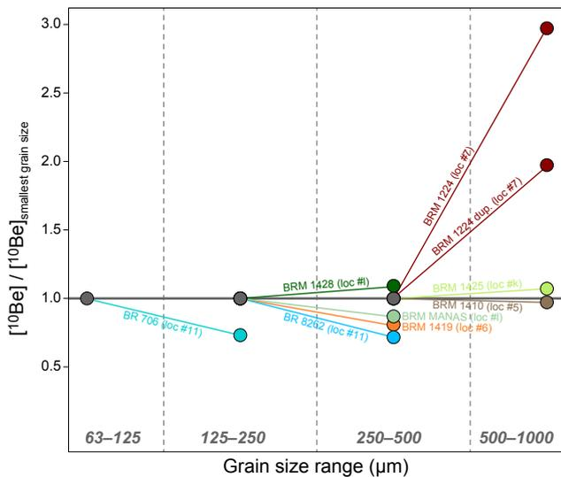
**Figure 2.** Ratio of  $^{10}\text{Be}$  concentrations from grain size pairs of the same sediment sample. Concentrations are normalized to the concentration of the lowest grain size fraction for comparison amongst samples.
